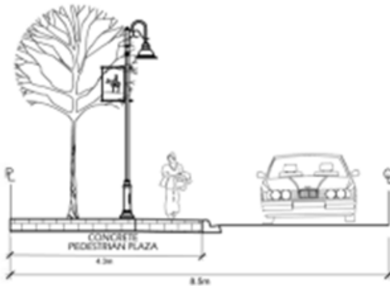
Figure 9: Typical Boundary Road Enhancement (Pedestrian Plaza)
