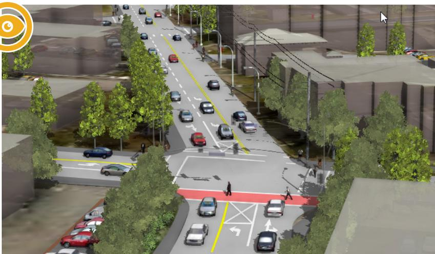
**Centre Avenue and First Street Intersection.** Two southbound lanes end. Right lane allows right turn access onto First Street W and southbound Centre Avenue thru traffic. Left lane becomes dedicated left turning lane onto First Street E.
