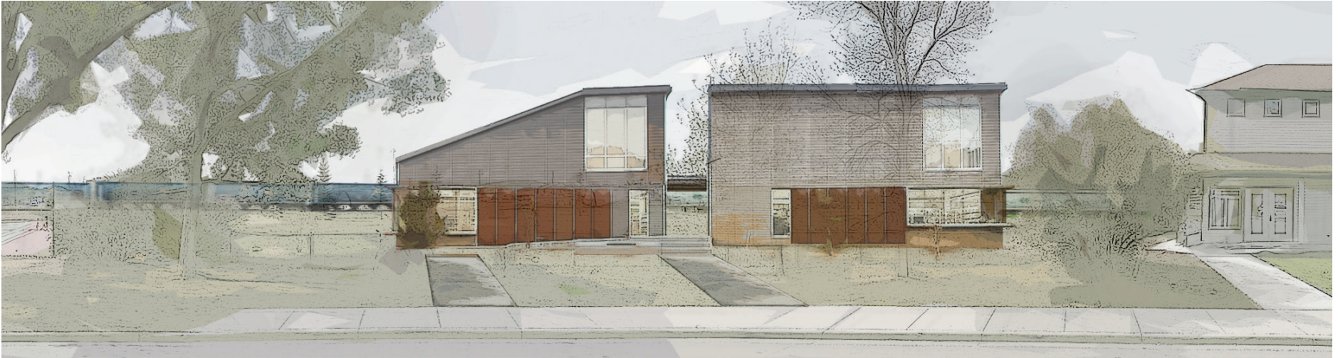
4.2.1(a) This sketched building has been sited and designed to offer framed views of the rail corridor. It also supports the character of the Railway Transition Zone through cladding materials that interpret the railway's industrial character. (Fig. 78: ERA 2020)
