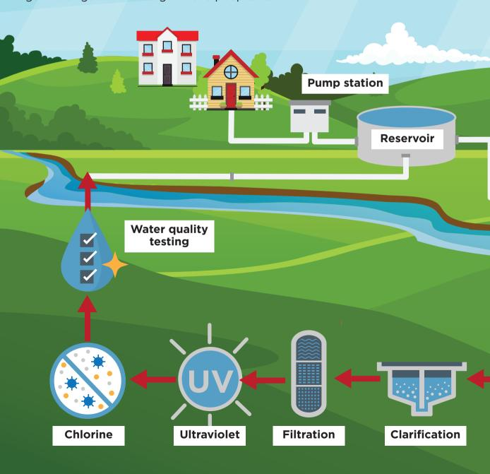
Before the water leaves the treatment plant, we add one more thing. A chemical called *chlorine* is added to make the water clean and safe to drink. The water gets around town and to your house through another set of underground pipes.
