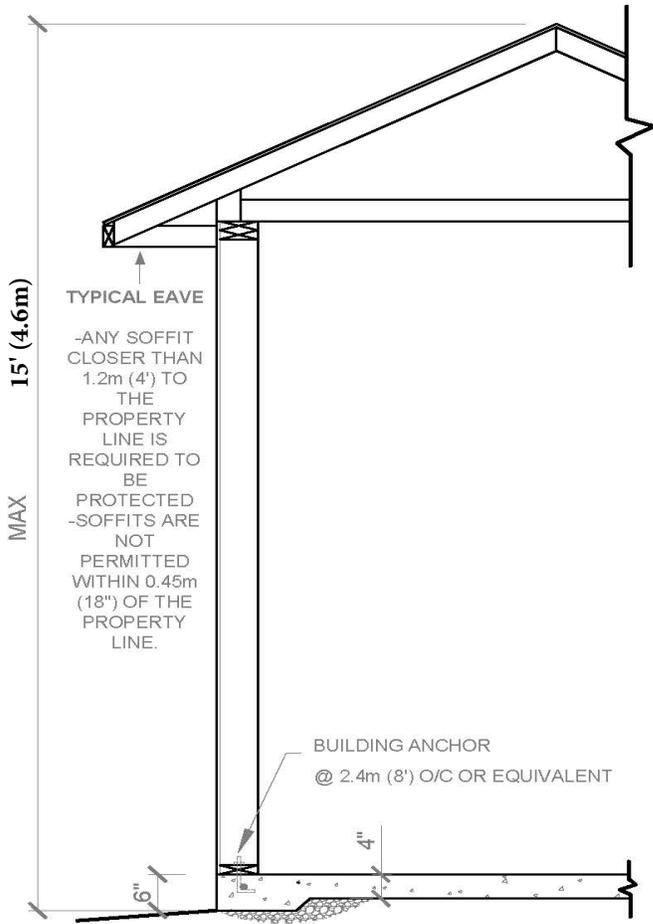
NOTE: ANY WOOD WITHIN 150mm (6") OF GRADE IS REQUIRED TO BE PROTECTED
