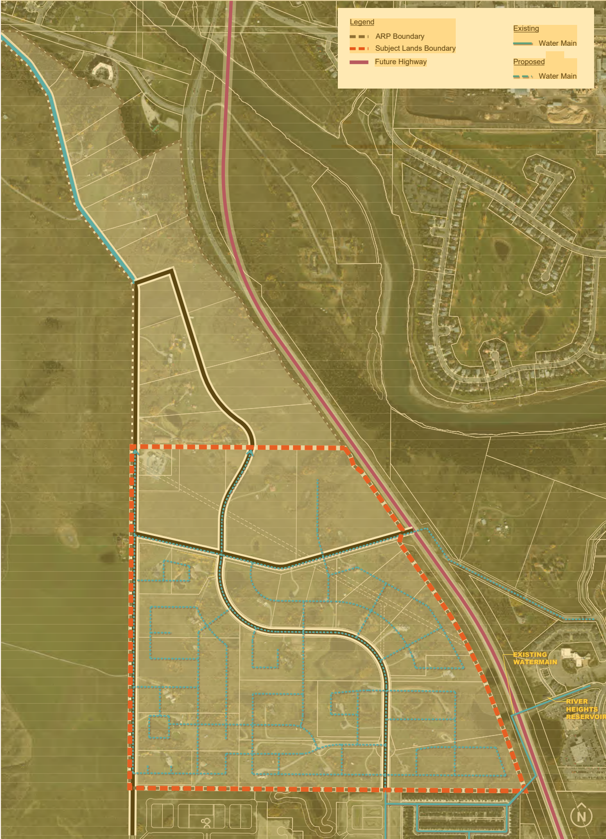
FIGURE 15: Servicing Network – Water
