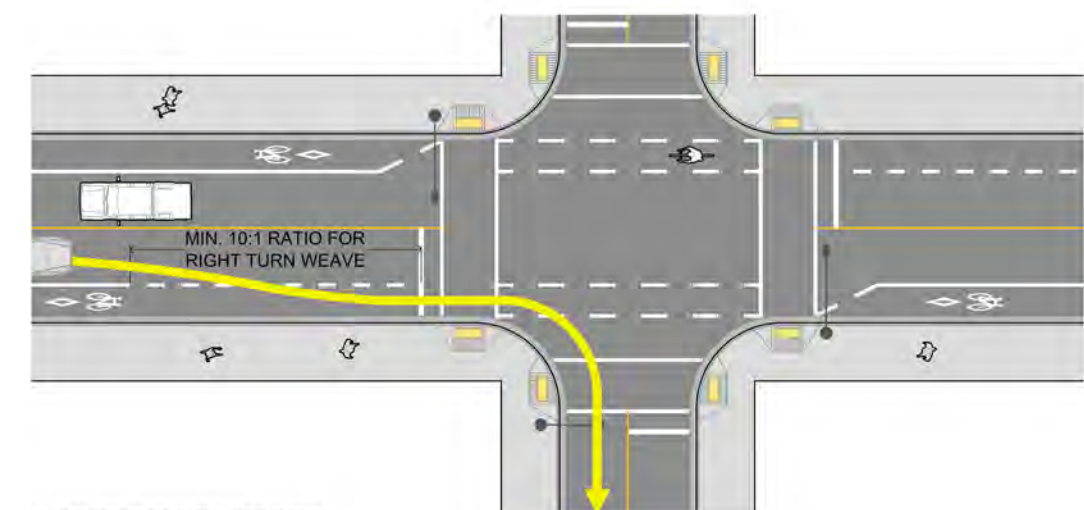
FIGURE 12 - CONTINUOUS BICYCLE LANE WITHOUT RIGHT TURN LANE
